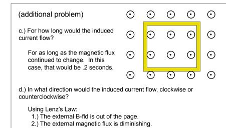
3.) As such, the induced B-fld must be in the same direction as the external flux. A current counterclockwise would produce the appropriate induced B-fld.
